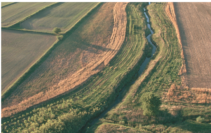
Figure 4. The trees and grasses in this filter strip trap sediment and other pollutants contained in runoff that could otherwise enter the stream. (Photo courtesy of USDA–NRCS.)
